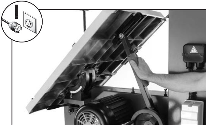
Figure 69. Lubricating table tilt rack and pinion assembly.
